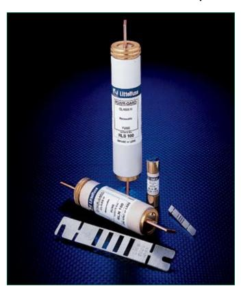
Littelfuse RLN/RLS series renewable fuses are a quality product that have traditionally been used to provide low cost protection of general purpose feeder and branch circuits where available short-circuit currents do not exceed 10,000 amperes. However, increased levels of available fault current and the possibility that renewable fuses may be improperly renewed is a potential safety hazard. In addition, escalating labor costs
